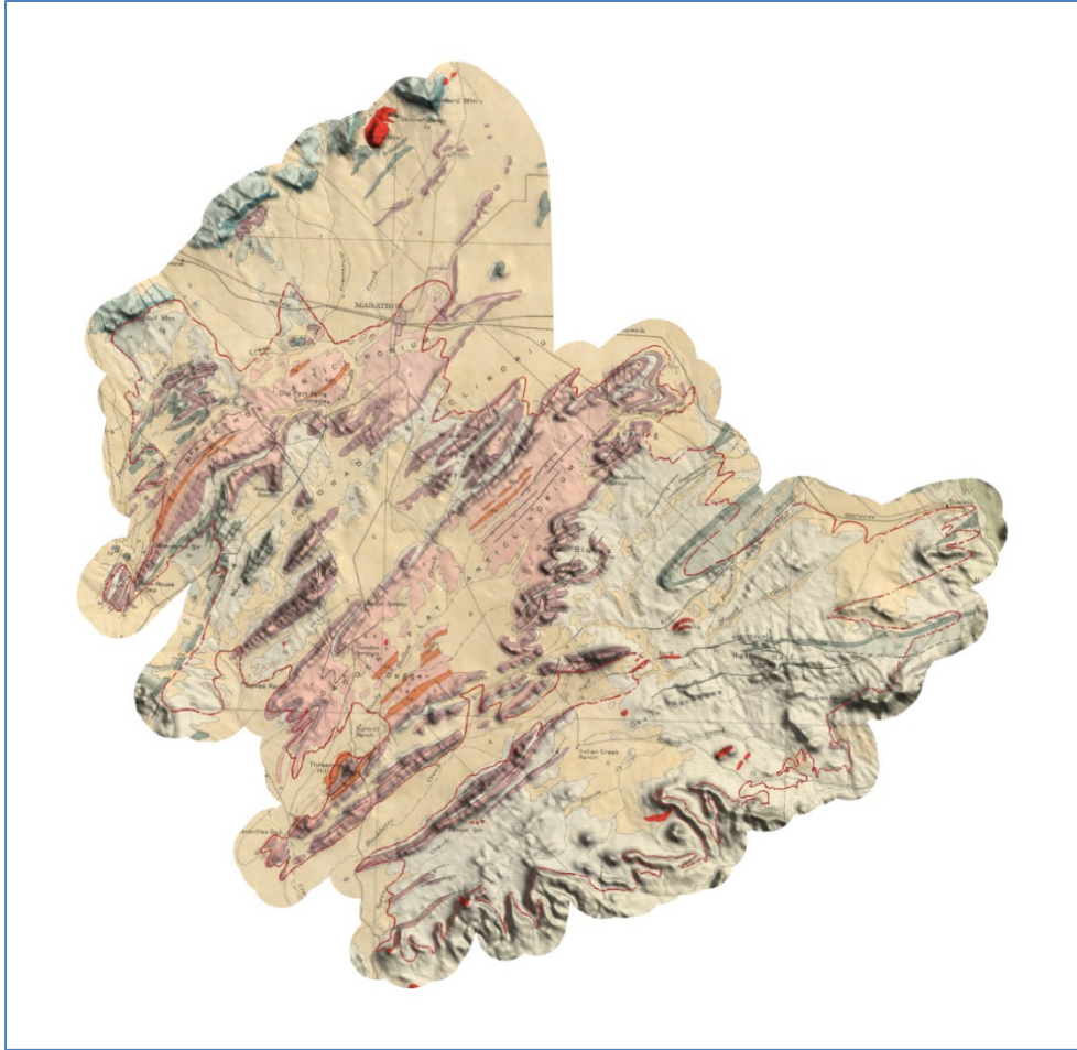
Figure 4-2. Extent of the Leapfrog model with a scanned map (Plate 23 of King, 1937) draped on a U.S. Geological Survey 30-meter digital elevation model. The extent of the Marathon Aquifer is shown as a red line.
